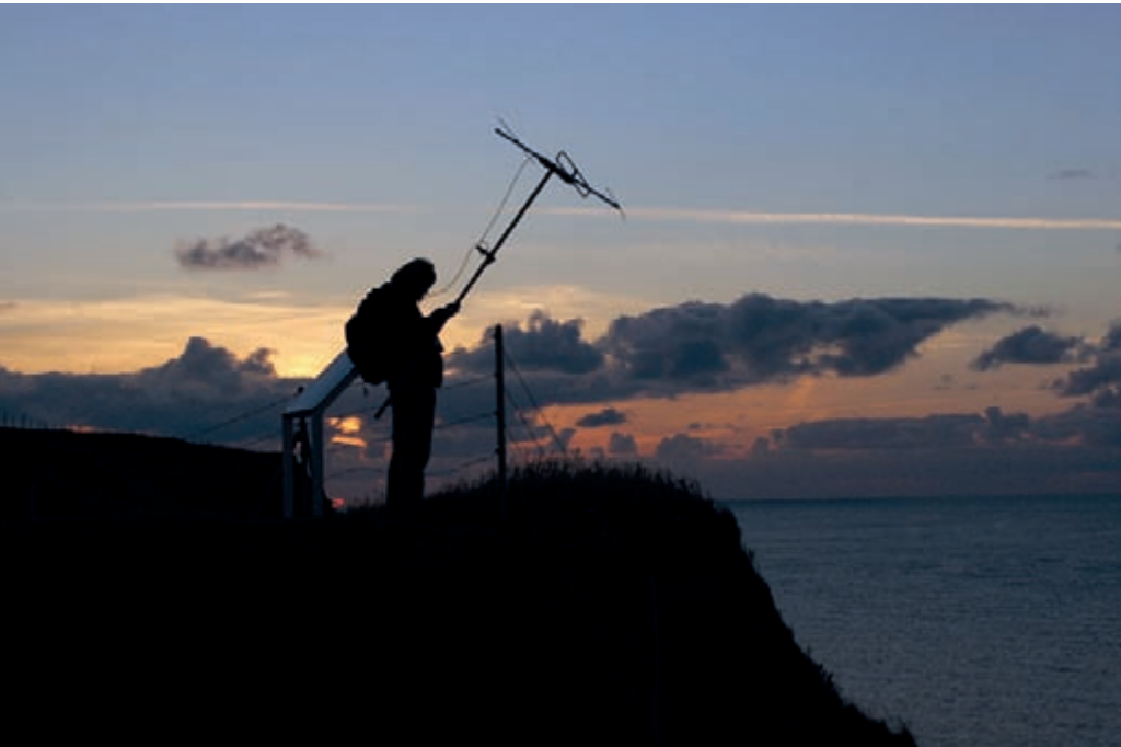
Radio-telemetry work at night on Helgoland. The radio antenna, together with a compass, is fastened to a pole so that the antenna does not need to be held all night long with outstretched arm; but also so that it can be held over the cliff edge to better locate the sleeping Northern Wheatears.
