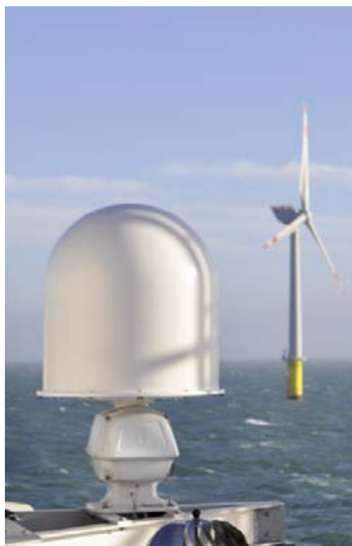
Marine radar with parabolic dish antenna covered by a radome for recording of migration direction at the offshore test field alpha ventus.
